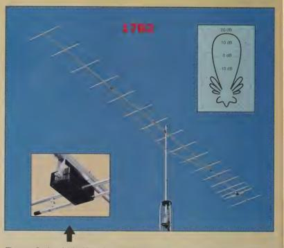
The new Cushcraft UltraMatch is a modified T-match system that provides a balanced current distribution on your Boomer. It uses UltraLink teflon® dielectric cable allowing for low loss high power applications. UltraMatch is completely enclosed for weather proofing. UltraMatch features an N-connector on the 17B2 and UHF SO239 on the 13B2. When all weather performance is important, you will choose the new UltraMatched Boomers everytime.
