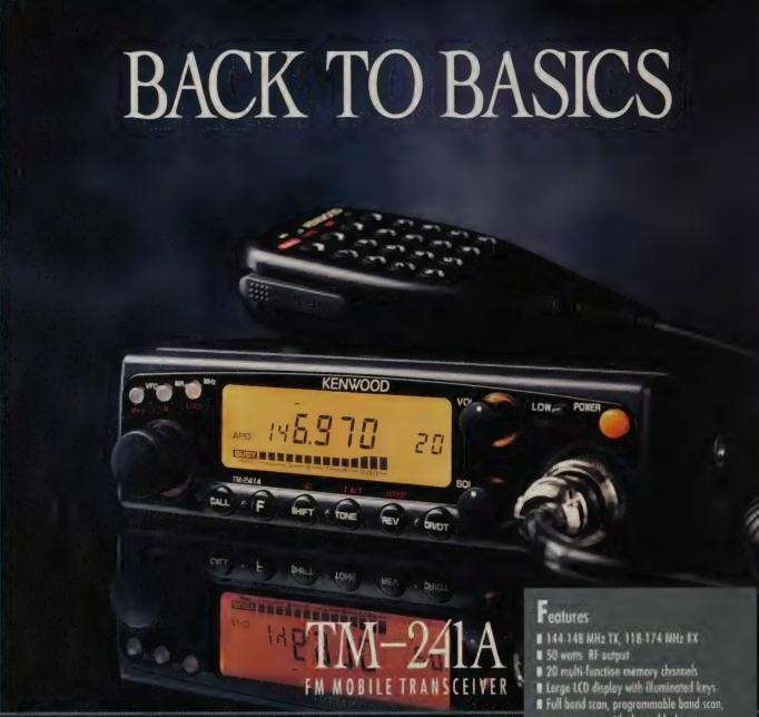
Pure and simple, the concept reads like this: "rock-solid performance with straightforward operation, at an affordable cost". And Kenwood's TM-241A (144MHz) FM mobile transceiver symbolizes this perfectly.
