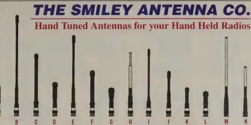
Each Smiley handheld antenna is individually hand tuned to resonance at band center under normal operating conditions. (No ground plane - No radials). Manufactured from the finest heat-treated copper plated spring steel coils. Cold rubber compound is used for coil insulation and a neoprene heat-shrink coating applied for strength and endurance. All have BNC connectors.
