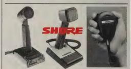
▶ 444D (left) A dual-impedance CONTROLLED MAGNETIC® fixed station microphone with a 200 to 6000Hz response, tailored for optimum speech intelligibility. Switch selectable for high  $(15k\Omega - 10M\Omega)$  or low  $(200-100\Omega\Omega)$  impedance inputs, and for Normal or VOX operation. Momentary or locking push-to-talk switch bar, 2% vertical height adjustment. Coiled three-conductor microphone cord, supplied with a wiring guide, requires proper connector. 2 lbs, 6 oz. **\$82**<sup>95</sup>
