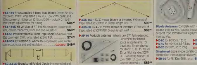
pretuned. Covers 3.5–30MHz continuous with VSWR less than 2:1. 52Ω coax feed, 90 ft long, rated 2KW PEP. Install as a hori \$17995 zontal flattop, an inverted-V, or sloper for DX...... **BWD 1.8-30** Same as AC 3.5-30 but covers 1.8-30MHz con tinuous. Rated at 2KW PEP, 90 ft. long .... \$179<sup>95</sup>
