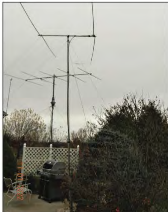
Bob, W3HKK, built this low-budget 10M Moxon Yagi just for the CQ WW contest. Who says you need big antennas to have fun?
